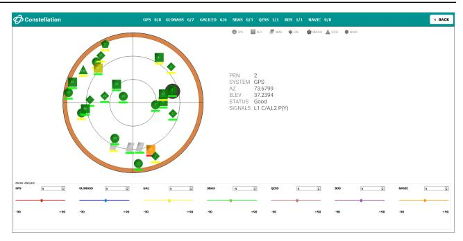
The satellites being tracked are represented with the following icons according to their satellite system:
