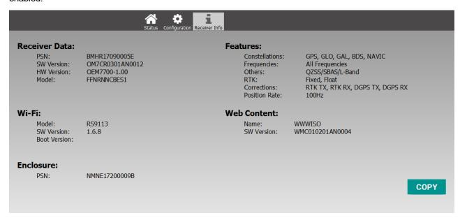
Click the **COPY** button to copy a VERSION log for this receiver into your computer's clip board. This log can then be pasted into any text editor. The VERSION log contains additional version information about the receiver Click the **Receiver Info** button again to hide the receiver information.
