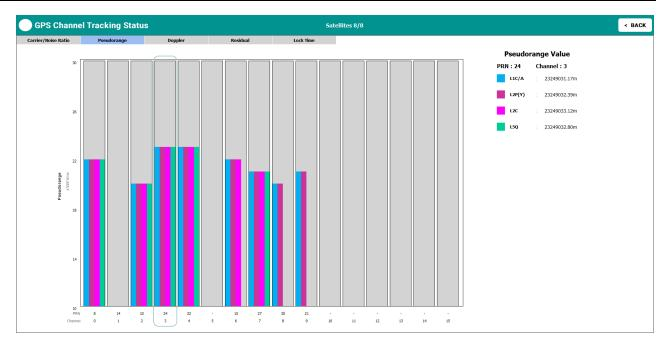
Pseudorange (km) values are displayed in this window. These values indicate the distance to the Satellite from the Antenna.
