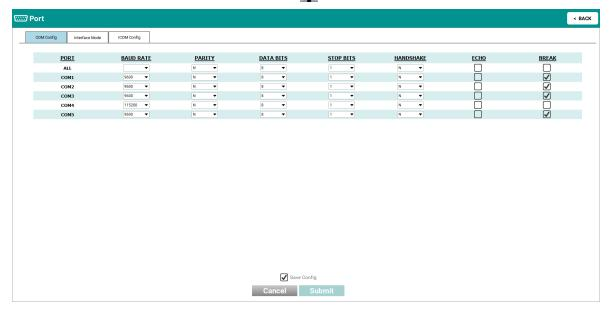
The *Port* configuration window shows the current COM port settings for each COM port available on the receiver.
