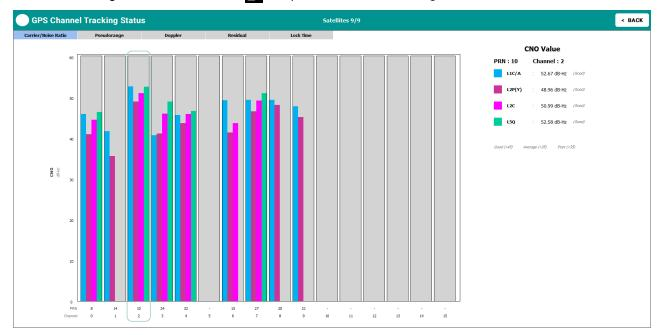
Carrier to noise density ratio (dB-Hz) values are displayed in this window. These values indicate the strength of the signal.
