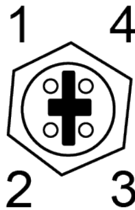
Figure 3: SMART7 Ethernet Connector (model dependent)
