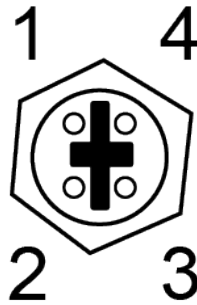
Figure 3: SMART7 Ethernet Connector (model dependent)
