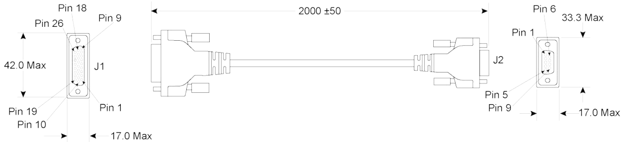
Figure 41: PwrPak7 COM1 Cable
