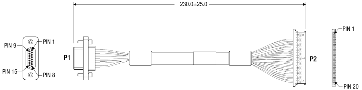
Figure 77: STIM300 IMU-to-MIC Cable Assembly
