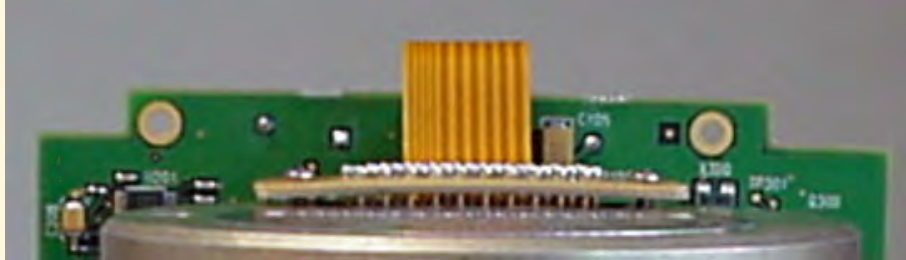
Figure 118: Correct (flat) flex cable installation
