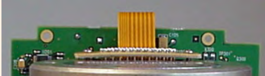
Figure 139: Correct (flat) flex cable installation
