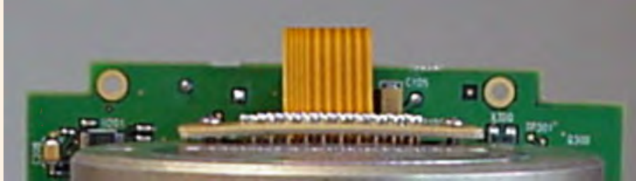
Figure 139: Correct (flat) flex cable installation
