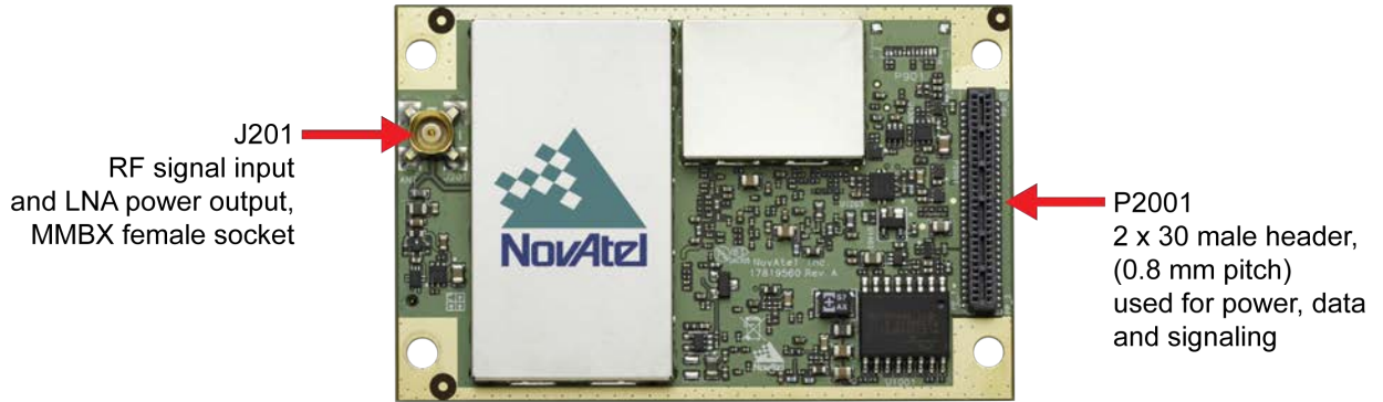
Figure 13: OEM7700 Connector and Indicator Locations
