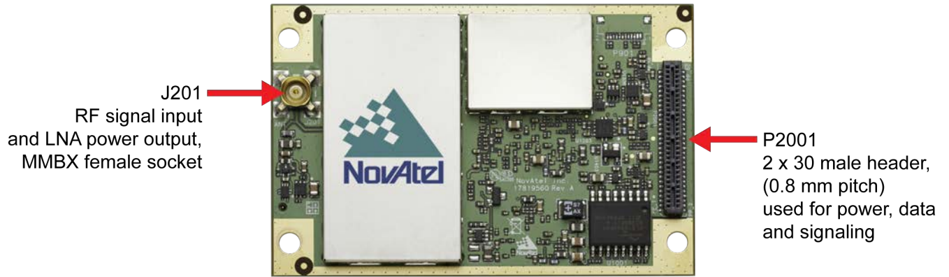
Figure 16: OEM7700 Connector and Indicator Locations
