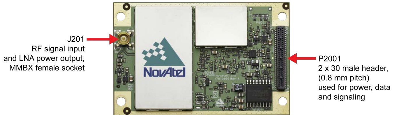
Figure 16: OEM7700 Connector and Indicator Locations
