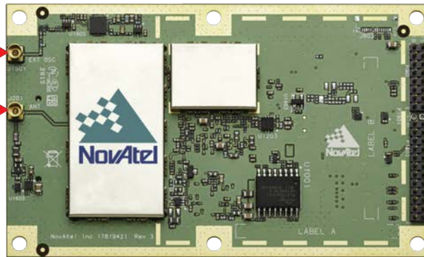
Figure 14: OEM729 Connector and Indicator Locations
