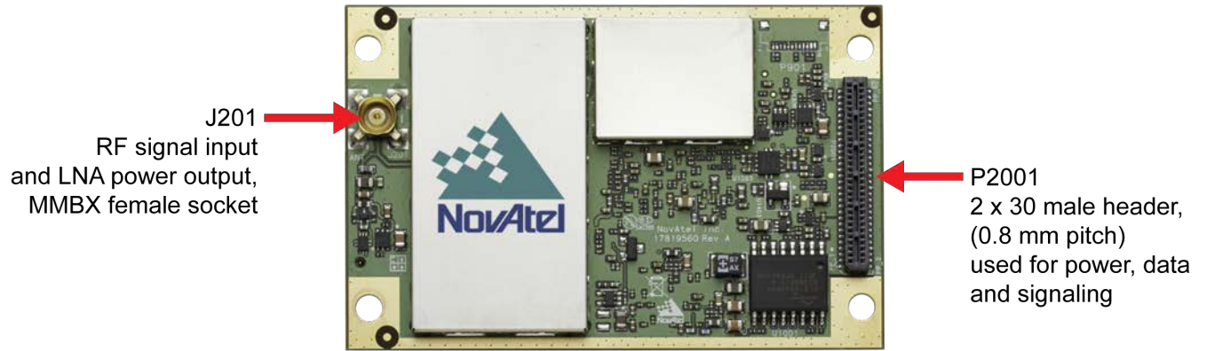
Figure 16: OEM7700 Connector and Indicator Locations
