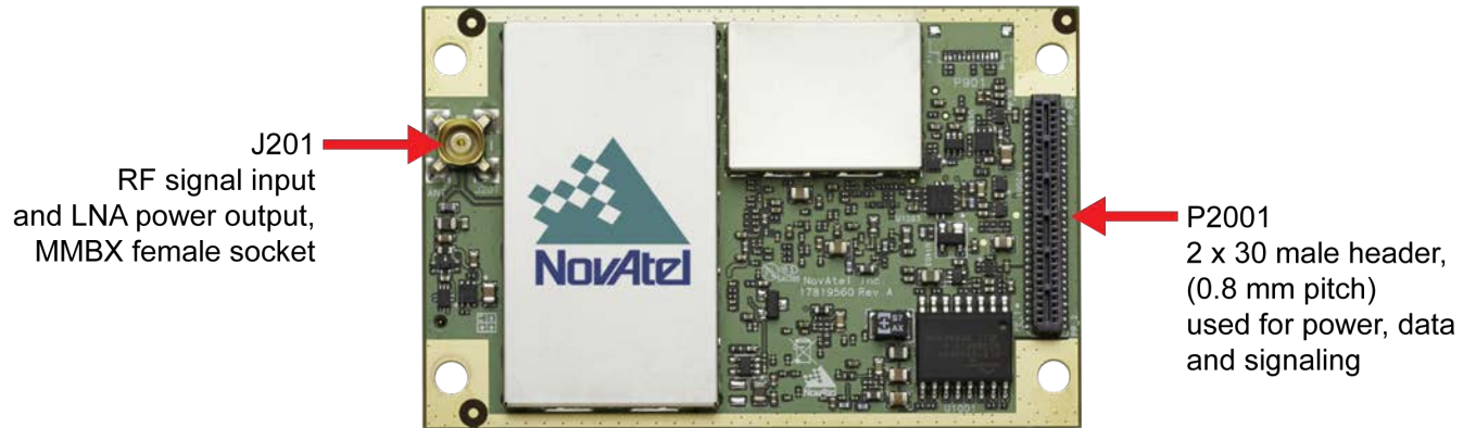
Figure 16: OEM7700 Connector and Indicator Locations
