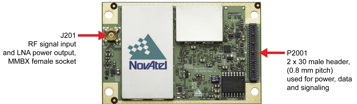
Figure 16: OEM7700 Connector and Indicator Locations
