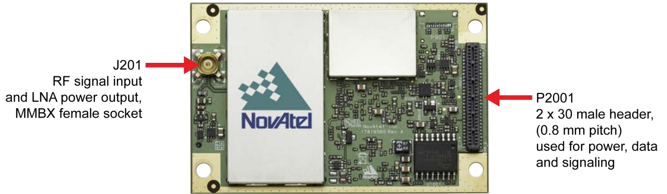
Figure 16: OEM7700 Connector and Indicator Locations
