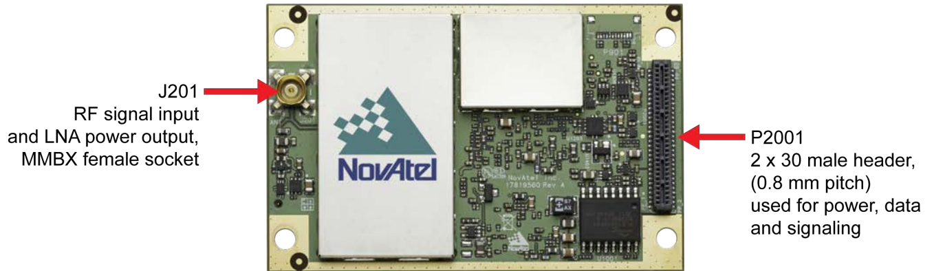
Figure 16: OEM7700 Connector and Indicator Locations
