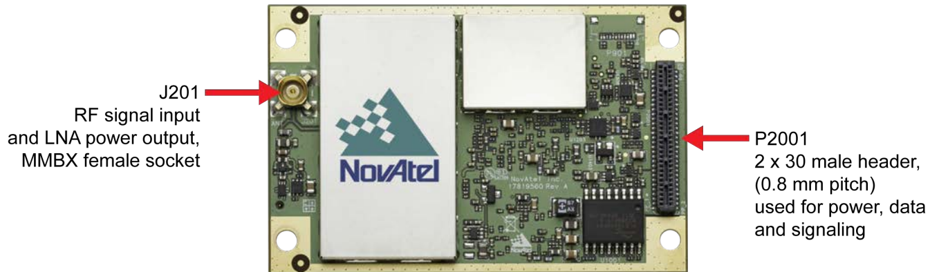
Figure 16: OEM7700 Connector and Indicator Locations
