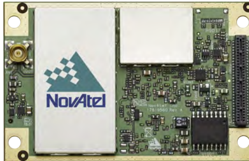
Figure 5: OEM7700 receiver board
