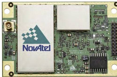
Figure 2: OEM719 receiver board
