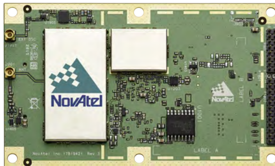
Figure 3: OEM729 receiver board
