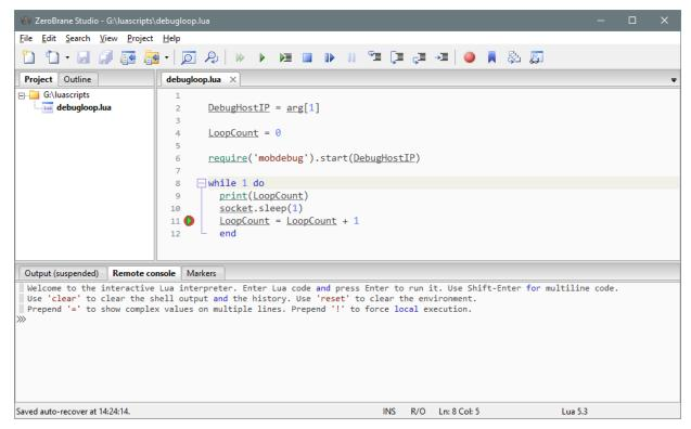
12. Use the debugging controls within the IDE to step through the code and set break points.
