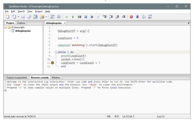
12. Use the debugging controls within the IDE to step through the code and set break points.
